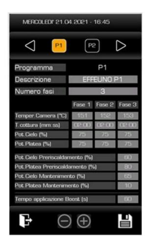
For each of the 30 programs it is possible to change the name (using an alphanumeric keypad that pops up on the screen), the number of phases and, as parameters, the upper/oven set-point temperature, the cooking time, the upper/floor percentages and the percentages to be used in the preheating and maintain mode.
