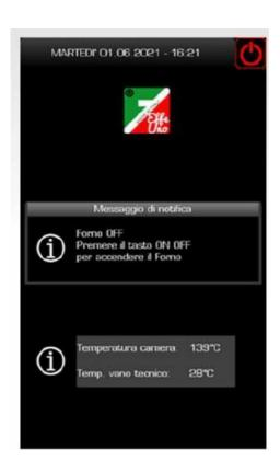
To turn the oven on, tap and hold the ON/OFF switch on the top right (for at least 4 seconds). In this way the oven will go into standby mode: it is now in operation but waiting for commands and the light is off. In fact, it will be in the 0 MANUAL program.
