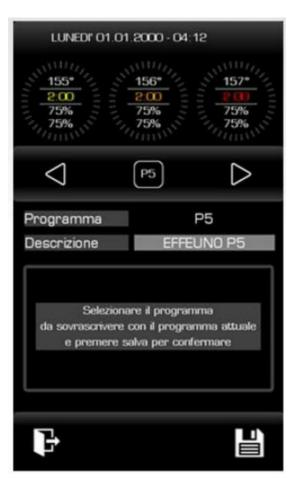
From this screen, it is possible to save the settings of the currently running program on one of the available programs (from 1 to 30). It is also possible to rename it with a maximum of 16 characters (using an alphanumeric
